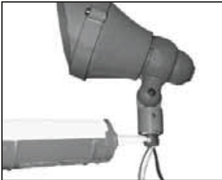
1. Coat threads with a good sealant.
